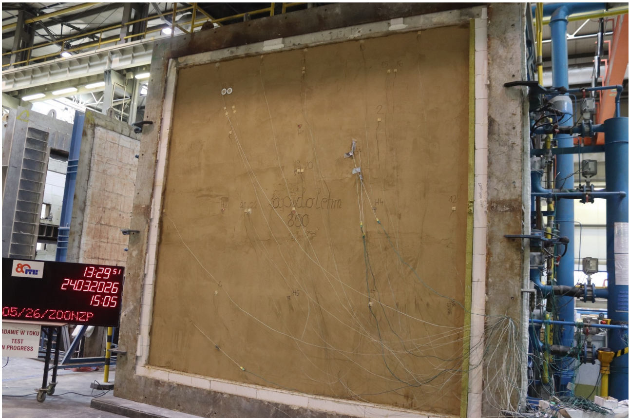
Fig. 13. Unexposed side of the test specimen, t = 15 \text{ min } 05 \text{ s}
