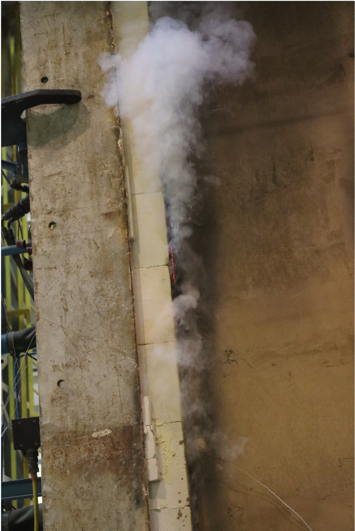
Fig. 19. Unexposed side of the test specimen, t = 120 \text{ min } 02 \text{ s}
