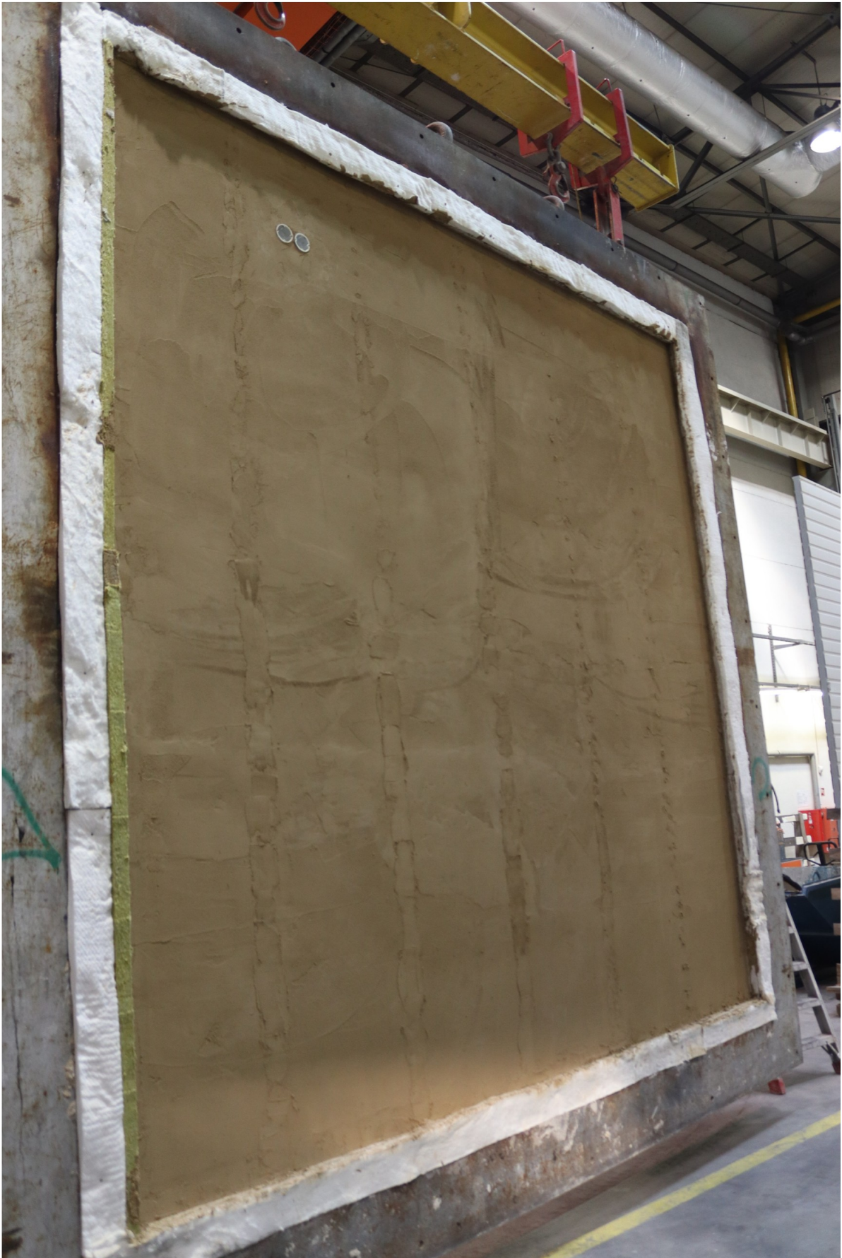
Fig. 2. Test specimen prior to the test - exposed side
