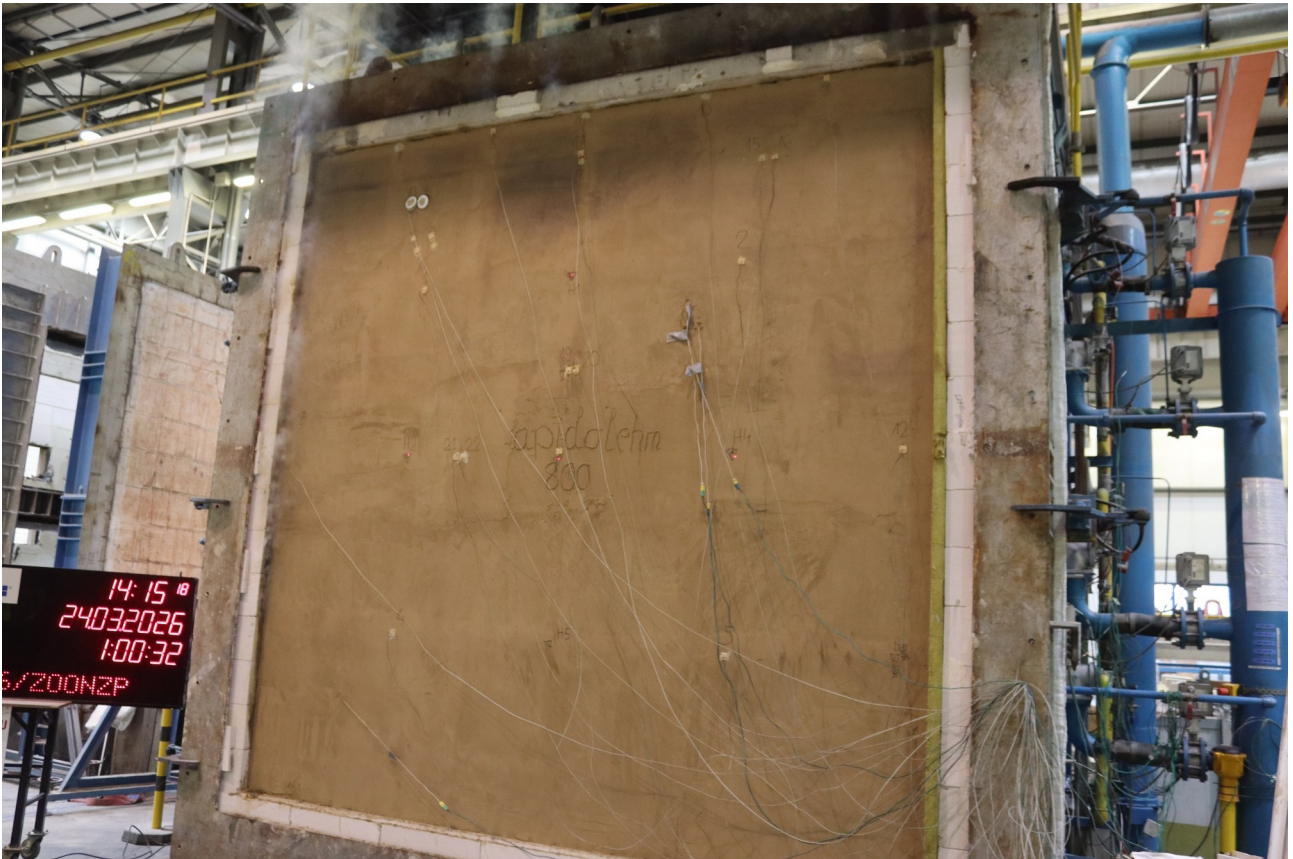
Fig. 15. Unexposed side of the test specimen, t = 60 \text{ min } 32 \text{ s}
