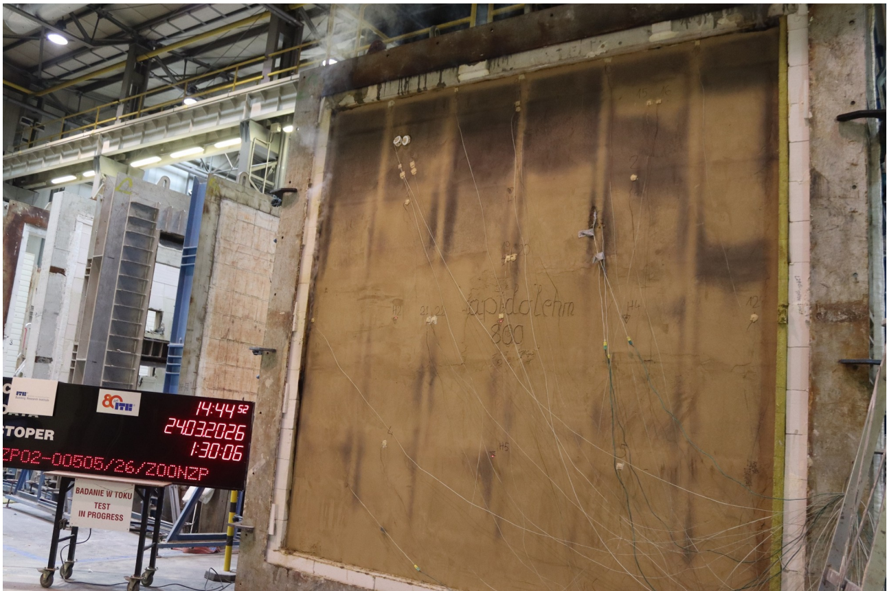
Fig. 17. Unexposed side of the test specimen, t = 90 \text{ min } 06 \text{ s}
