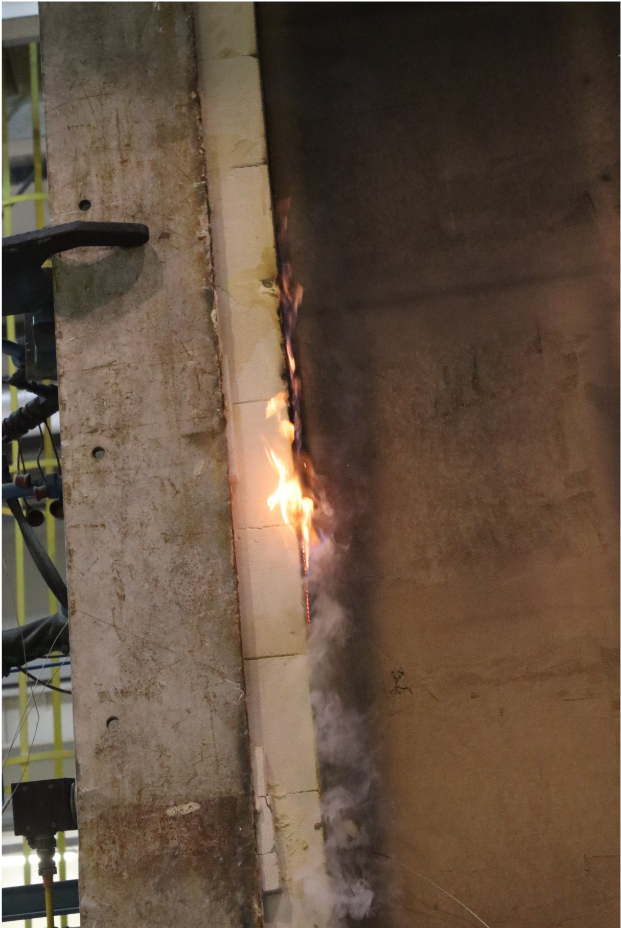
Fig. 20. Unexposed side of the test specimen, t = 121 \text{ min } 01 \text{ s}
