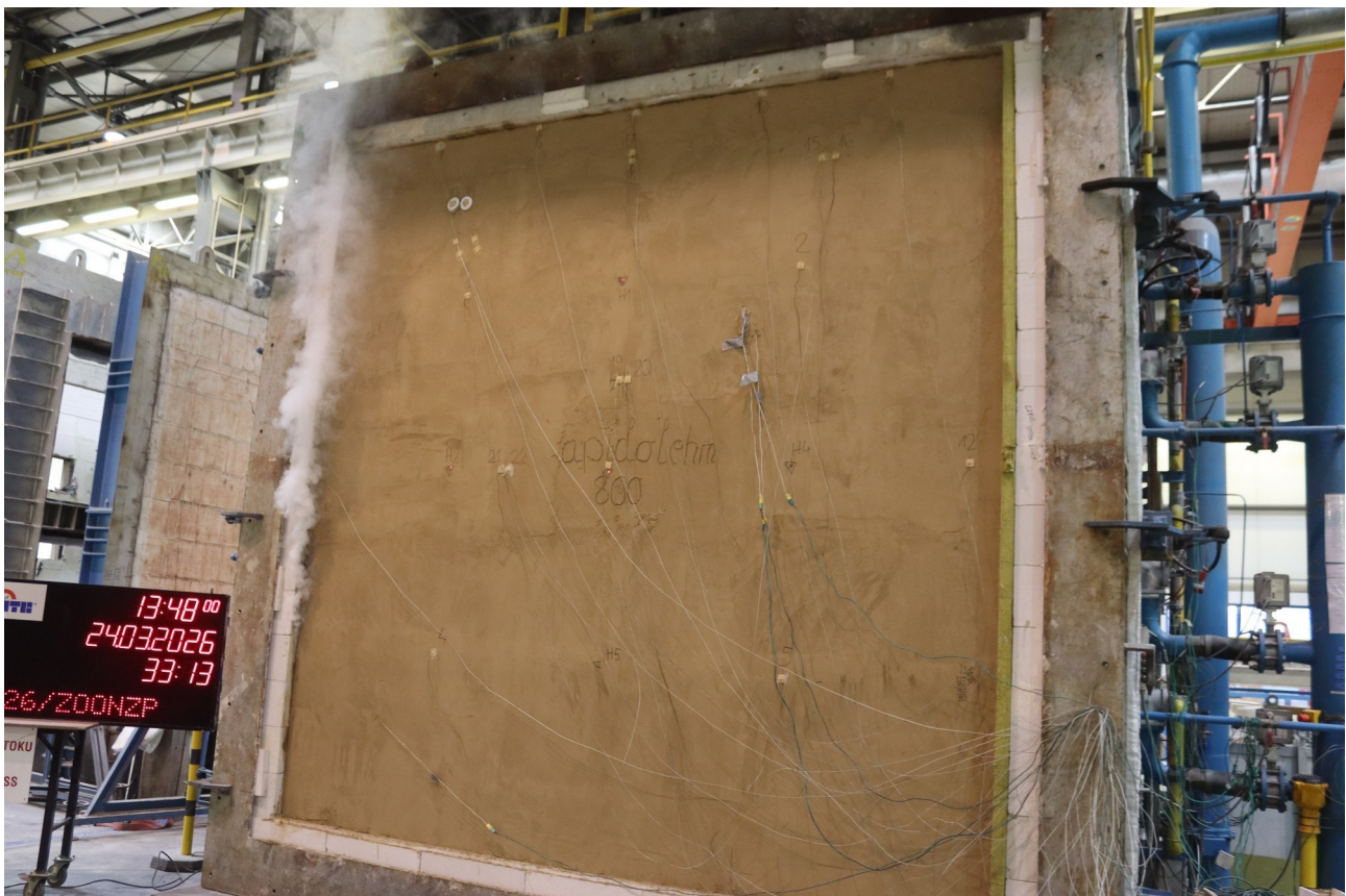
Fig. 14. Unexposed side of the test specimen, t = 33 \text{ min } 13 \text{ s}
