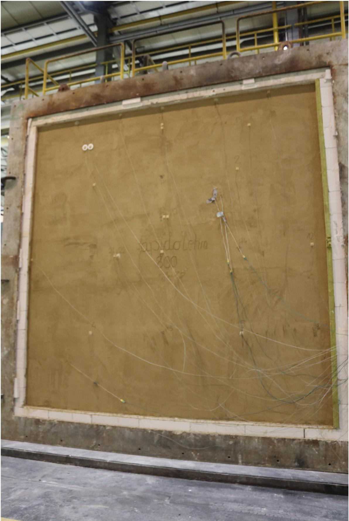
Fig. 1. Test specimen prior to the test - unexposed side
