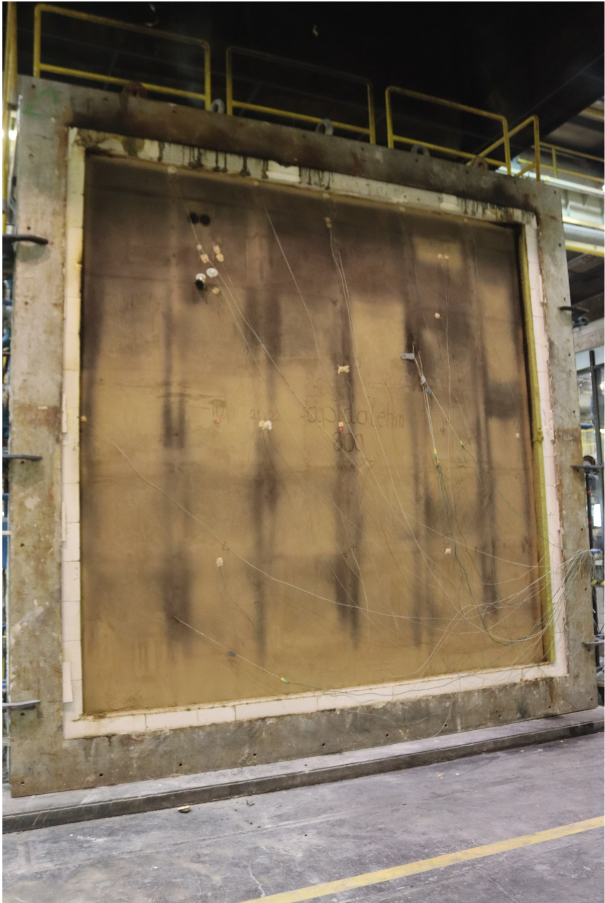
Fig. 22. Unexposed side of the test specimen just after termination of the test
