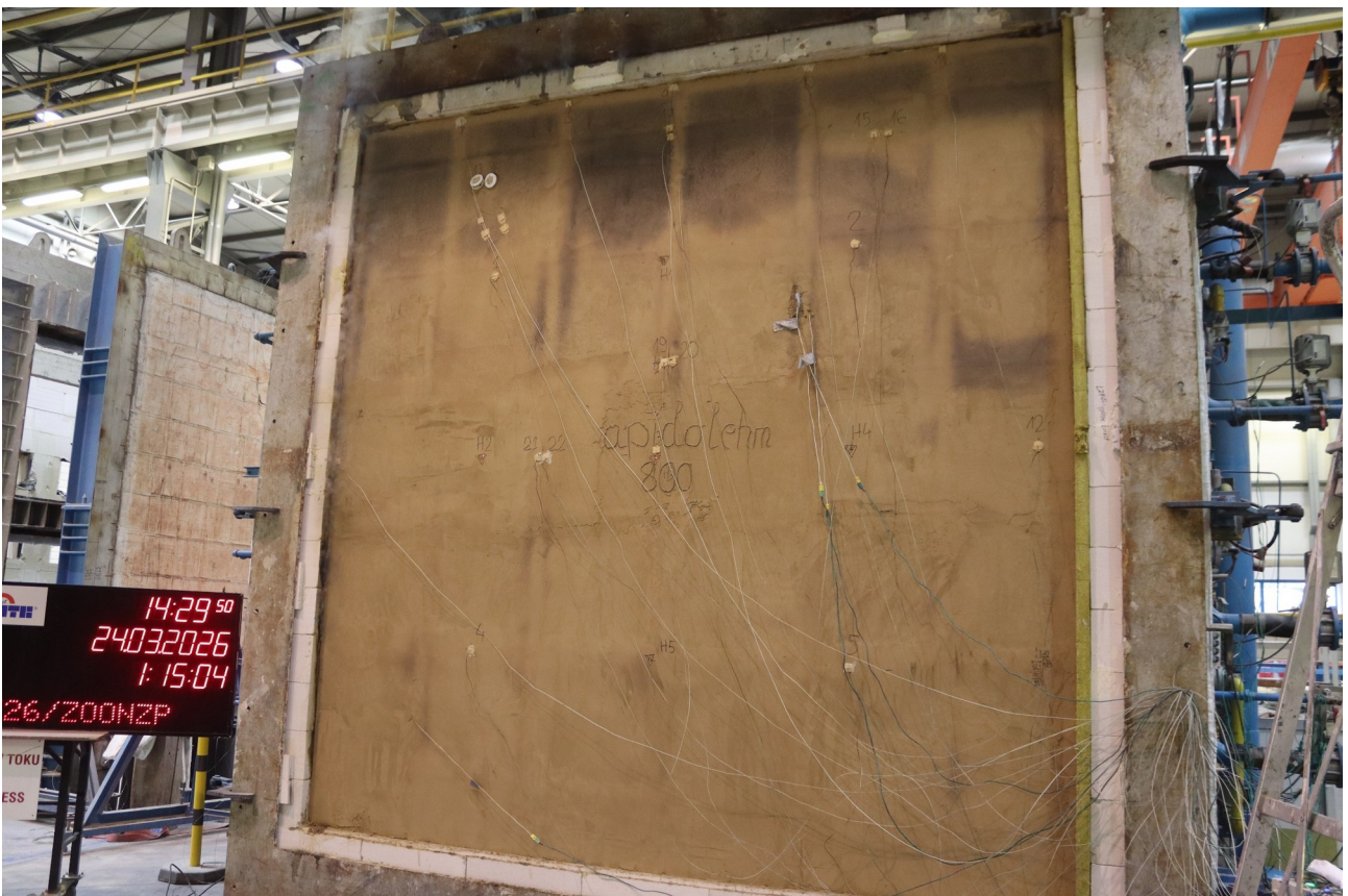
Fig. 16. Unexposed side of the test specimen, t = 75 \text{ min } 04 \text{ s}
